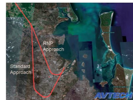
RNP procedures introduced at Brisbane reduced the 70 dB and 75 dB footprints, and allowed the procedure to be placed over non-residential areas such as the Brisbane River according to AVTECH.
